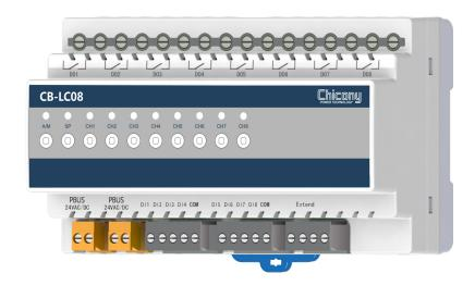
CB-LC08 is one of the relay control modules in the CB series which is widely used in the electromechanical equipment control field such as intelligent lighting and security alarm. It is equipped with functions of 8 digital input channels and 8 relay output channels; the digital input can receive signals of switches, alarm devices, and infrared sensors, etc. The relay output can control the switch circuit of the lighting, electric machinery, and alarms.
