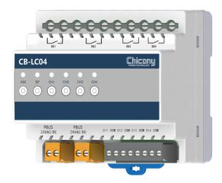
CB-LCO4 is one of the relay control modules in the CB series which is widely used in the electromechanical equipment control field such as intelligent lighting and security alarm. It is equipped with functions of 4 digital input channels and 4 relay output channels; the digital input can receive signals of switches, alarm devices, and infrared sensors, etc. The relay output can control the switch circuit of the lighting, electric machinery, and alarms.
