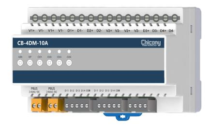
CB-4DM-10A is one of the dimming control modules in the CB series which is widely used in the field of intelligent lighting, smart homes, and room control. It is equipped with 4 channels of digital input and the dimming output function with 4 channels of 10A LED constant voltage. This function is applicable to conditions where various equivalent LED lights are in parallel connection and the digital input can receive signals of switches, alarm devices, and infrared sensors, etc.
